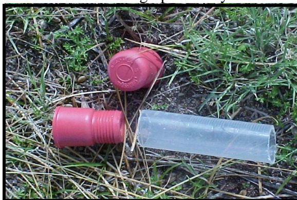
Soil Off-Gassing Collection Tubes
